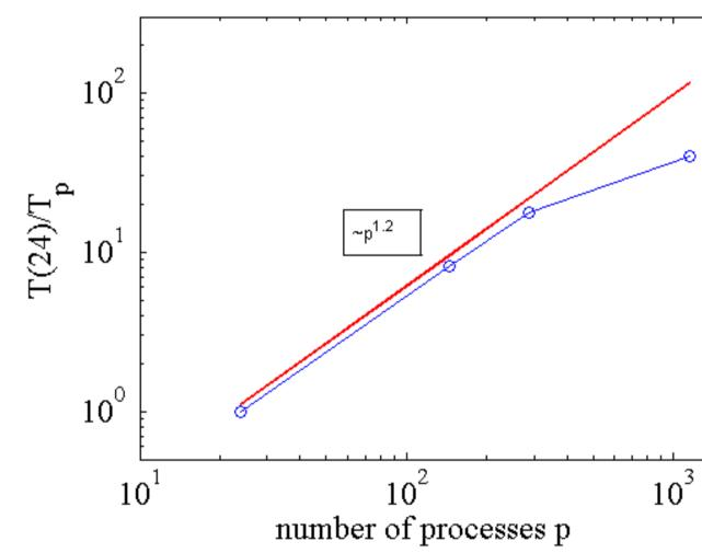
Strong scaling study for a 257x145x153 grid run for 5,000 timesteps using the parallel NetCDF I/O
