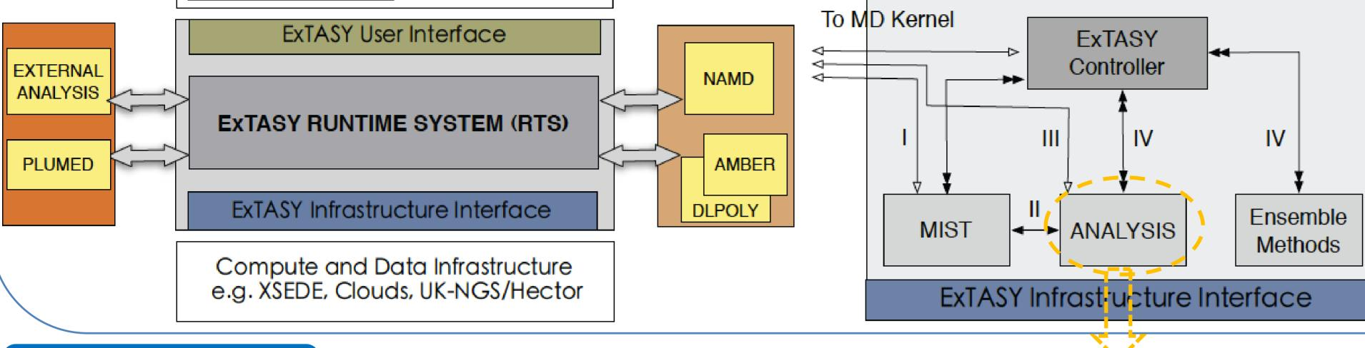
(B) Architecture for the **ExTASY Runtime**, which defines the main components and the control flow between them. Closed double-headed arrows represent communication between components internal to ExTASY; arrows with open-heads represent communication from an ExTASY component to the MD Engine. ExTASY uses SAGA-based Pilot-abstractions to provide fundamental support for ensembles, and SAGA to implement the infrastructure interface to different back-end systems.
